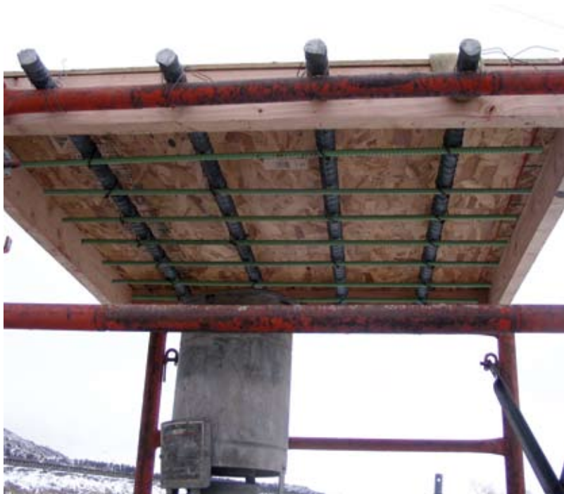
Project No. 1: Core grading test panel from Hoover Dam bypass bridge project
