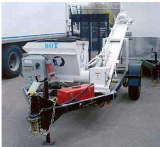
Predampener used in dry-mix shotcrete application
