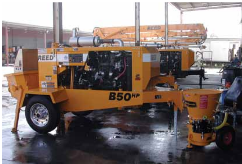
Wet-mix B50HP shotcrete pump (left) and dry-mix Lova shotcrete (gunite) gun (right)
