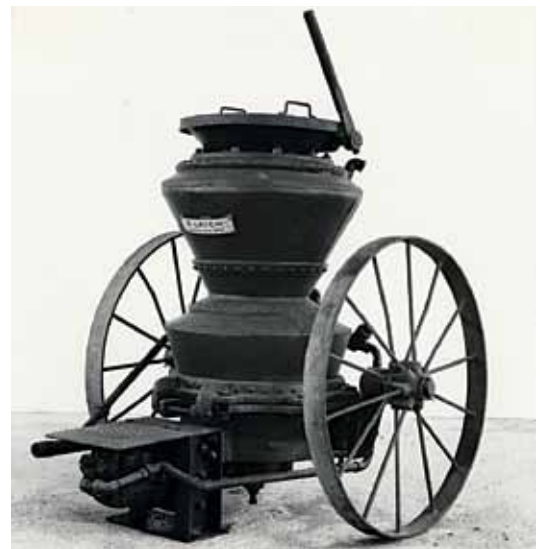
Fig. 2: Double-chamber gun (Cement-Gun, 1914)
