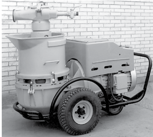
Fig. 3: Screw-type gun (Spribag BS-12, around 1950)
