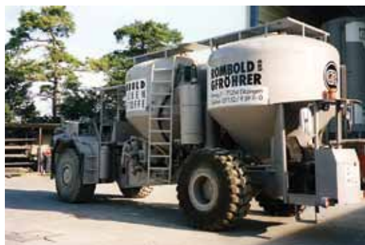
Fig. 8: Double pressure cylinder on truck, with bottom-mounted batching screws (Rombold-Spritzmobil, 2002)
