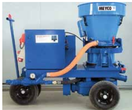
Fig. 7: Rotating-barrel gun (Meyco GM 090, 2002)
