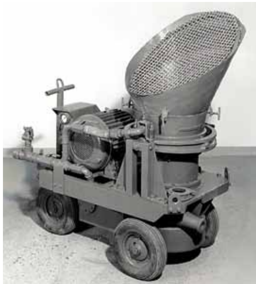
Fig. 5: Rotating-barrel gun (Meyco GM 57, No. 1)
