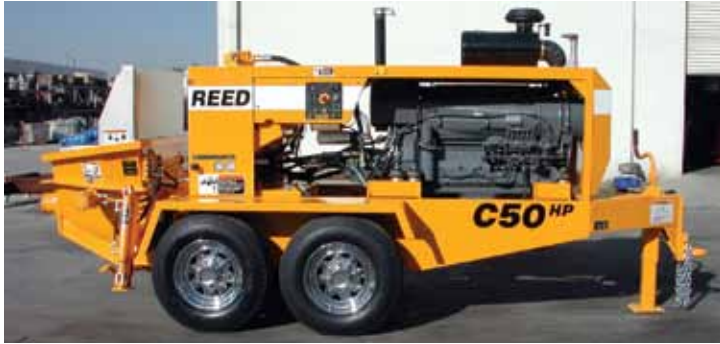
Fig. 4: A REED C50HP concrete pump
