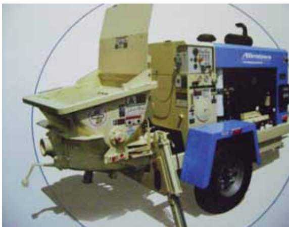
Fig. 6: An Allentown Powercreter 40 pump with hydraulic outriggers
