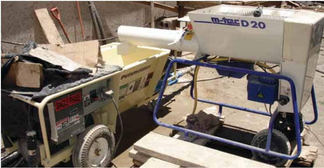
Fig. 1: An S 5 electric version rotor/stator unit with an M-Tec continuous mixer feeding it. This electric mixer comes with an adjustable water meter and low water-pressure cutoff that maintains a steady, consistently blended material flow
