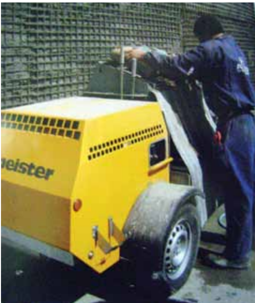
Fig. 2: The SP 13 high-pressure piston pump. The low profile gives the operator an unobstructed view of the work area and shooting area while making a batch of wet-mix concrete
