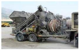
Fig. 5: Contractor-built gunite rig using auger mixing
