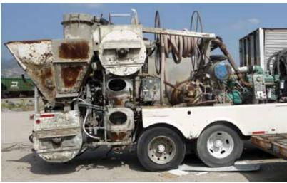
Fig. 2: View of the paddle mixer showing the double chamber gun
