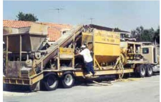
*Fig. 6: Self-contained gunite rig*
