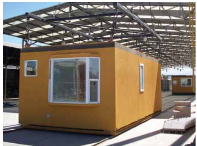
A fully finished Uni-Crete Cell housing module ready to ship to site
