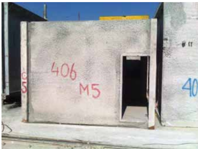
A Uni-Crete-Cell™ module ready for the assembly line
