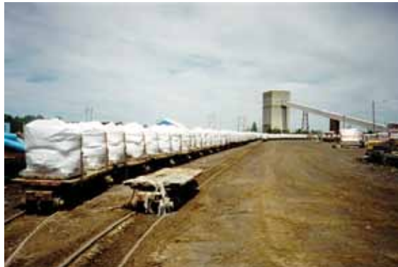
Fig. 3: Large, 2200 lb (1000 kg) bulk bags that allowed more material to be moved more quickly throughout the mine
