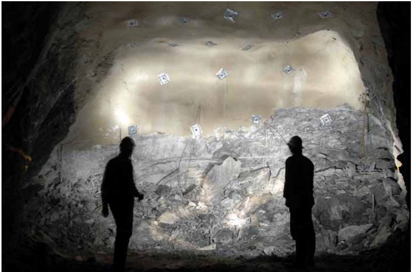
Fig. 2: Smooth, clean, and free of debris: mining with FRS and bolts
