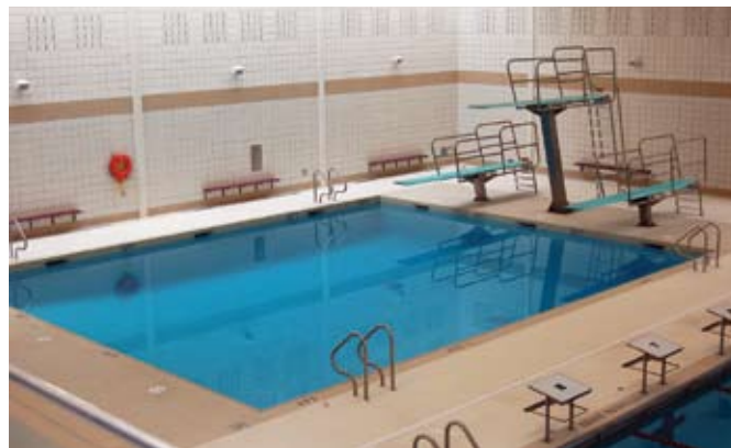
The 8 to 13 ft (2.4 to 4 m) deep pool with two 3 ft (0.9 m) diving stations and one 10 ft (3 m) diving station
