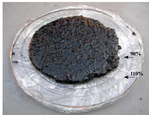
Fig. 2: Self-flow test for the R2U MgO-C castable
