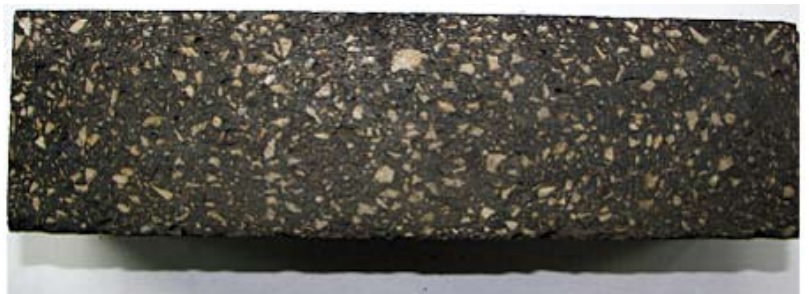
Fig. 1: Cross section of the novel R2U MgO-C castable
