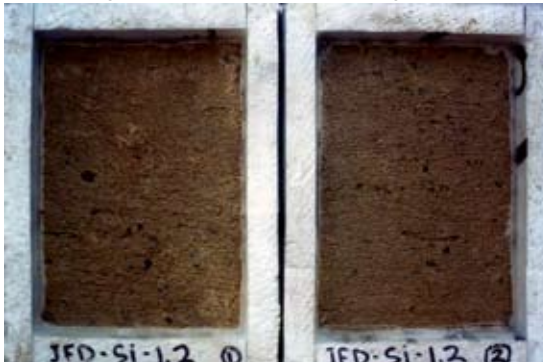
Fig. 2: Non-air-entrained versus air-entrained dry-mix shotcrete—air void system, ASTM C457 (60 \times magnification) and salt scaling resistance, ASTM C672
