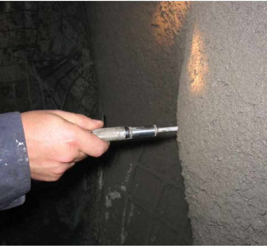
Fig. 12: Initial set time measurement
