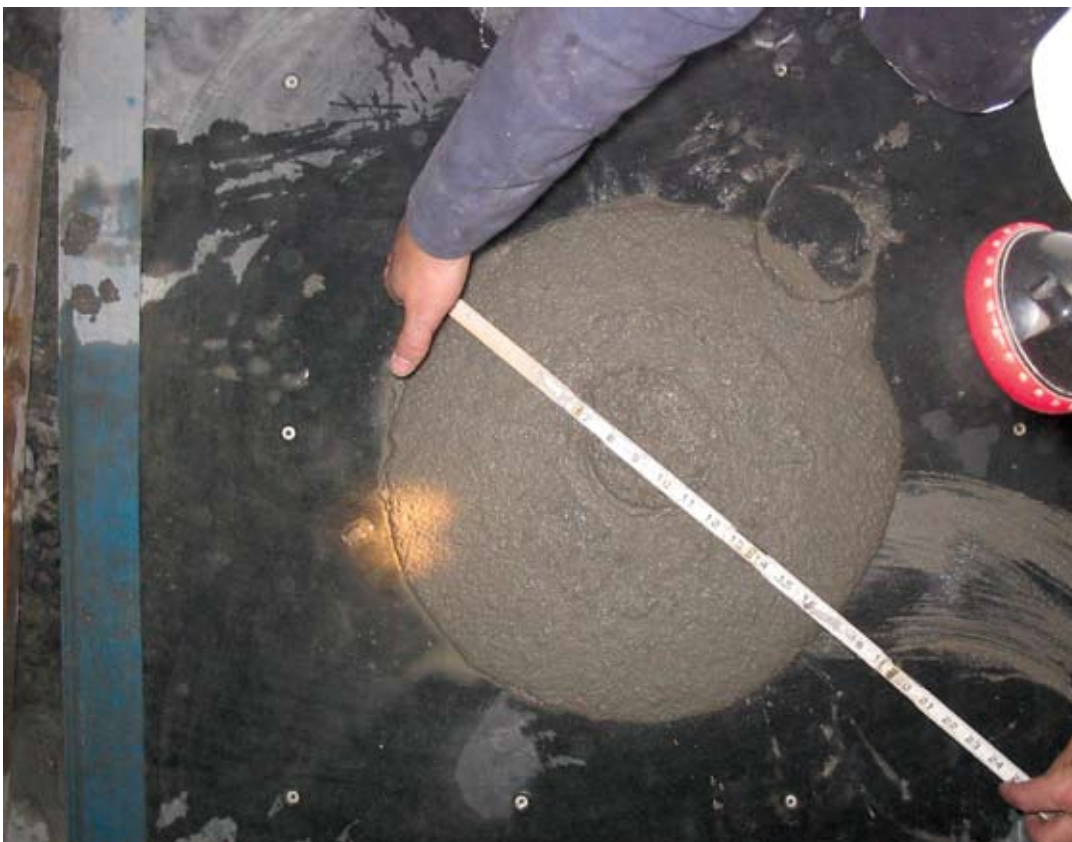
Fig. 11: Slump-spread of shotcrete mixture of 16.5 in. (419 mm) underground
