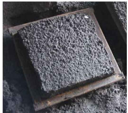
Fig. 13: Shotcrete panel for determining the compressive strength
