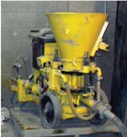
Fig. 1 : Dry-mix shooting gun and nozzle
