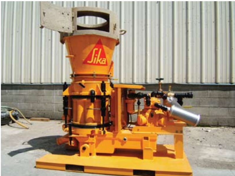
Shotcrete machine with enclosed hopper hood
