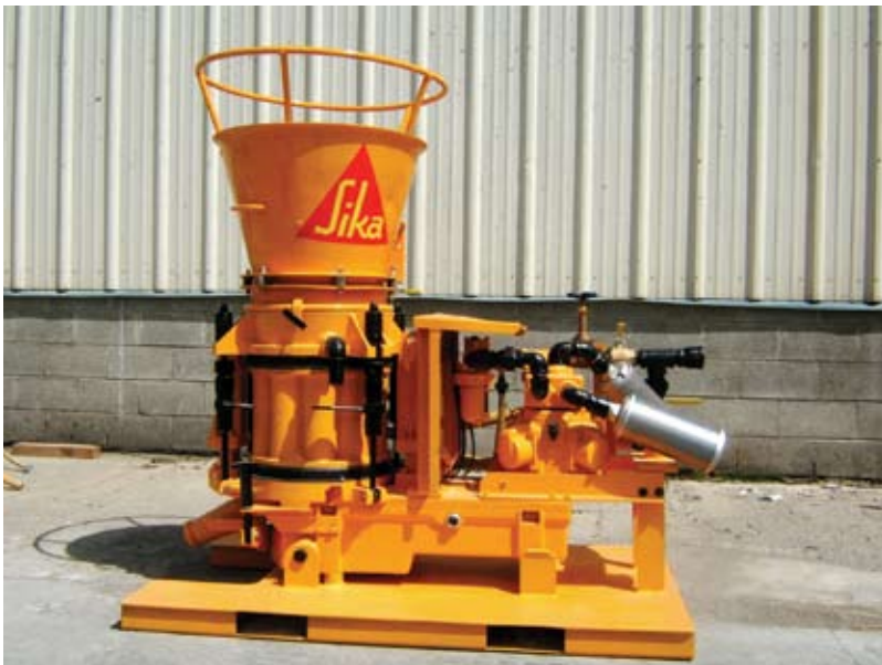
Shotcrete machine with open hopper guard
