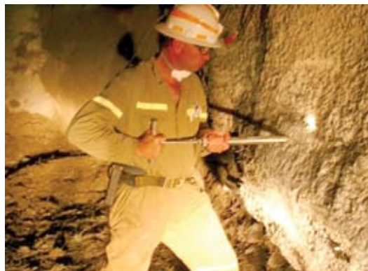
Fig. 2: Early strength test with a Meyco Penetrometer
