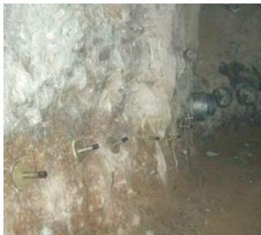
Fig. 7: Pull-out discs in underground mine
