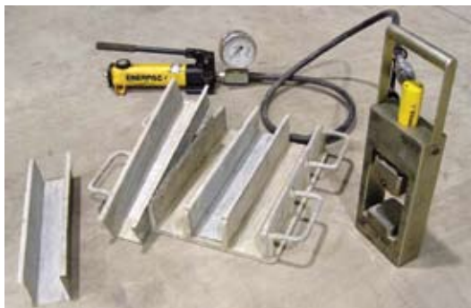
Fig. 3: Beam end tester (right) with mold and sheet steel inserts
