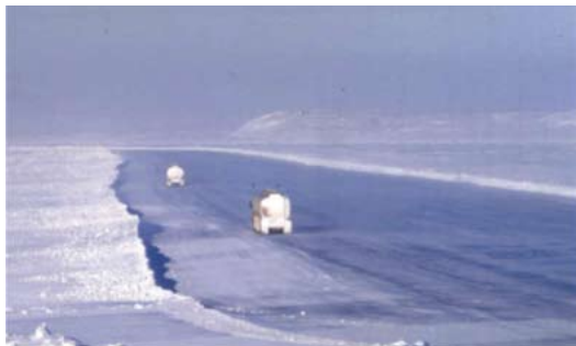
Fig. 1: Trucks moving material to the site over the "ice road"
