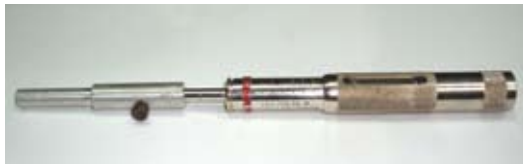
Fig. 7: Portable penetrometer measuring plastic dry-mix shotcrete consistency
