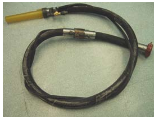
Fig. 5: Hydronozzle (water ring inserted 10 ft [3 m] from nozzle tip)
