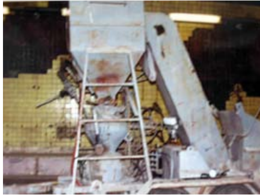
Dry-process shotcrete machine with premoistener
