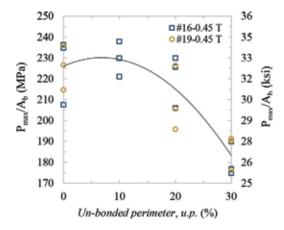
Fig. 8—Effect of u.p. on ultimate bond stress of bars No. 16 (No. 5) and No. 19 (No. 6).
