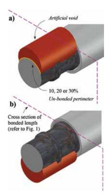
Fig. 3—(a) Top; and (b) bottom position of artificial voids.
