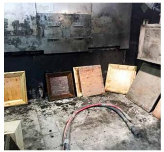
Fig. 2: Conventional square shotcrete test panels used for obtaining cores
