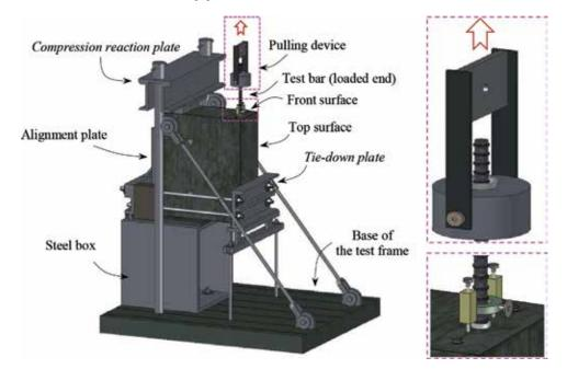
Fig. 5—Test setup of ASTM A944-10 "beam-end" specimen.
