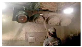
Fig. 6: Shotcrete being sprayed into inclined AASHTO T 344 rings
