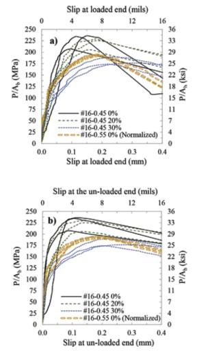
*Fig.* 13—(*a*) *Stress-slip curves of* 0.45 *and* 0.55 w/b *mixtures at loaded; and (b) unloaded end.*
