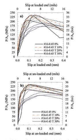
Fig. 6—(a) Stress-slip curves of No. 16 (No. 5) test bars at loaded; and (b) unloaded end.
