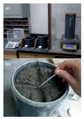
*Fig.* 4—(*a*) *Equipment needed for bleed test; and (b) bleed water collected from container.*
