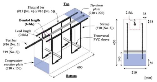
*Fig. 1—ASTM A944-10 "beam-end" specimen. (Note: 25.4 mm = 1 in.)*
