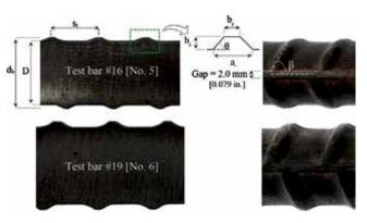
Fig. 2—Longitudinal cut with geometry nomenclature of No. 16 (No. 5) and No. 19 (No. 6) bars.
