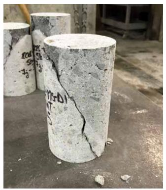
Fig. 5: Composite core for slant shear bond strength testing (ASTM C882/C882M)
