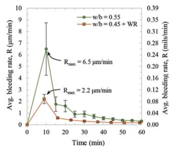
*Fig. 11—Average bleeding rate of mixtures. (Note: 1 \mum/min = 0.039 mils/min.)*
