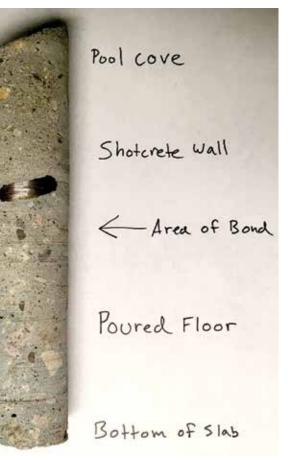
Fig. 6: Core demonstrating excellent bond of shotcrete to a poured floor
