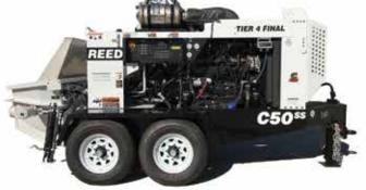
REED'S C50SS Shotcrete Pump is EXTREMELY POWERFUL (225HP 6.7 Liter 6 Cylinder Cummins) and SUPER SMOOTH (Closed-Loop Hydraulics (2000 psi, Variable Stroke Speed))
