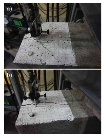
Fig. 14—(a) Y-; and (b) T-shape splitting patterns at front surface (grids are  $15 \times 15 \text{ mm} [0.6 \times 0.6 \text{ in.}]$ ).
