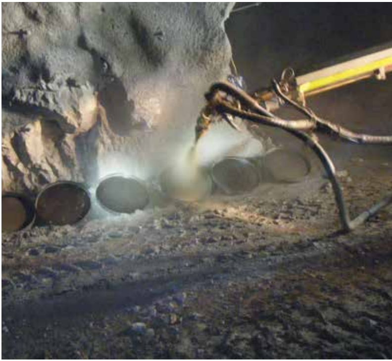
Fig. 8: ASTM C1550 toughness panels being sprayed at underground site
