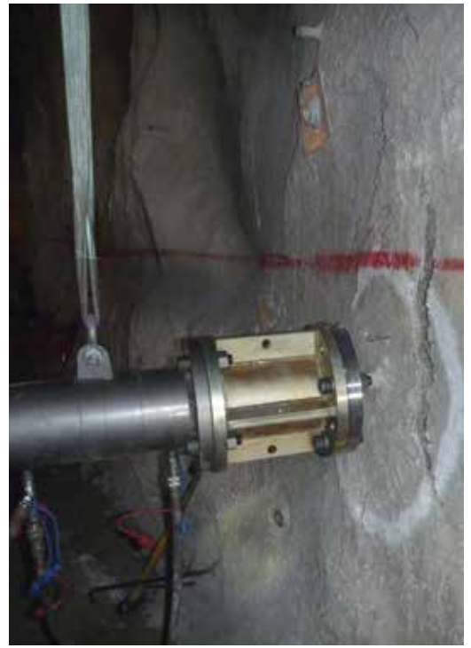
Fig. 9: Large-scale shotcrete capacity test
