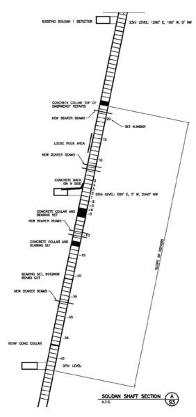
Fig. 2: Elevation view of the shaft repair area
