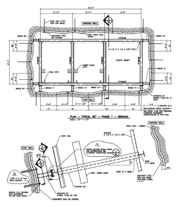
Fig. 1: Plan and profile section of the shaft repair (Note: 1 in. = 25.4 mm; 1 ft = 0.328 m)
