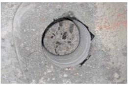
*Fig. 6: A hole after a core has been extracted during a pulloff test*
