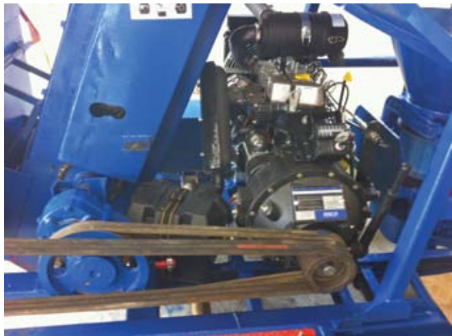
Allentown R900 Batch Rig refurbish with a conversion from air motor to diesel motor
