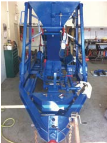
Allentown R900 Batch Rig refurbish before conversion from air motor to diesel motor
