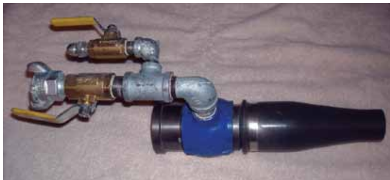
Fig. 2: ACME nozzle with integrated air/accelerator port
