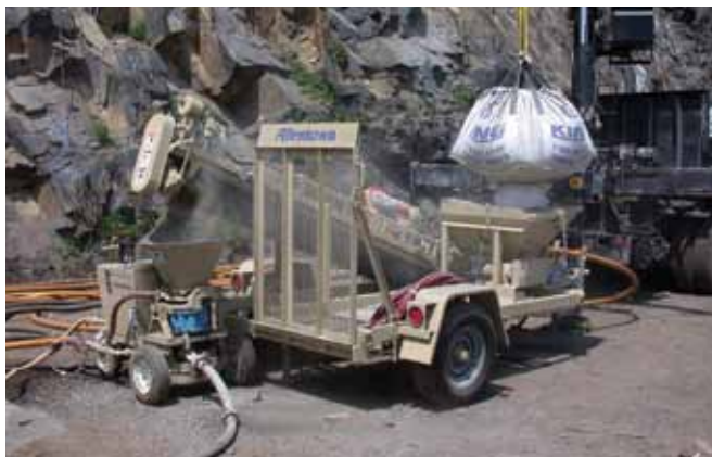
Predampening equipment should be used to reduce the amount of airborne dust at the machine and at the nozzle
