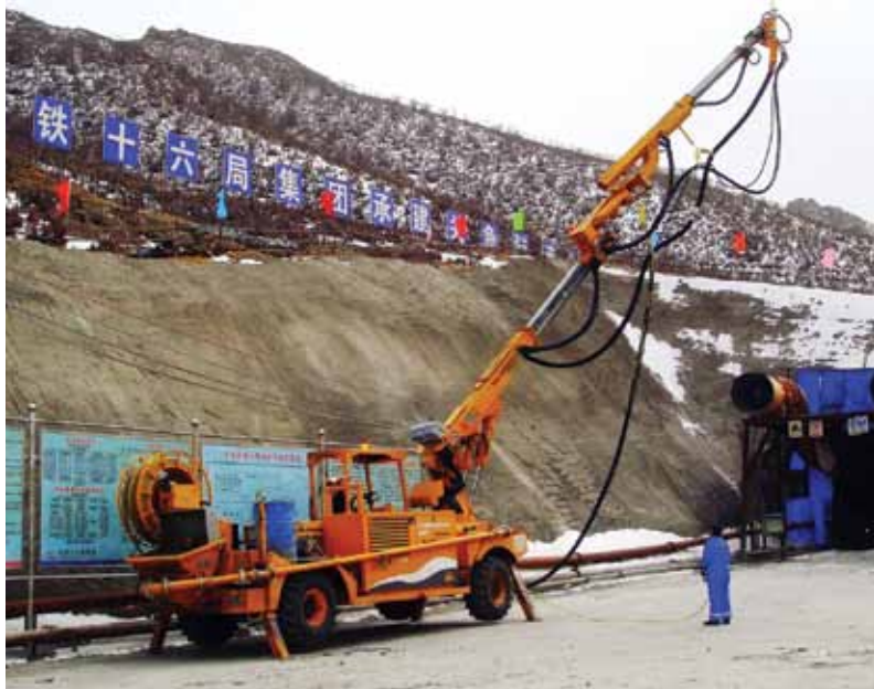
This operator familiarizes himself with the remote control of the modern concrete-spraying system
