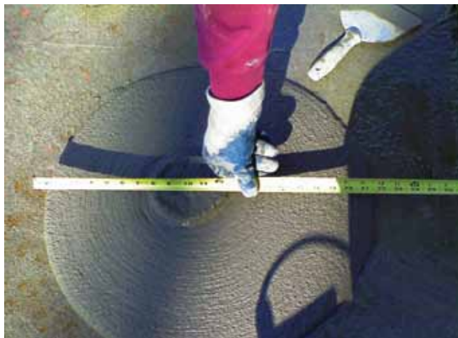
A 22 in. (559 mm) slump-spread shotcrete mixture
