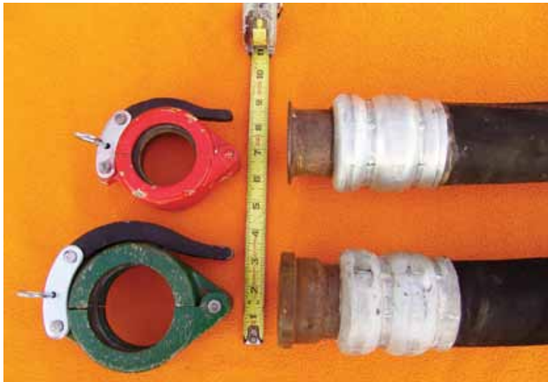
Fig 4: Heavy-duty coupler (bottom) weighs nearly 40% more than the flared end fitting (top). Both have a 2 in. (50 mm) interior diameter
