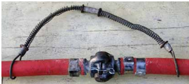
Fig 7: A Chicago-style fitting with whip check and safety clip in place
