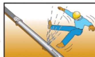
Figure 7 Delivery system components must be able to withstand maximum pump pressure
