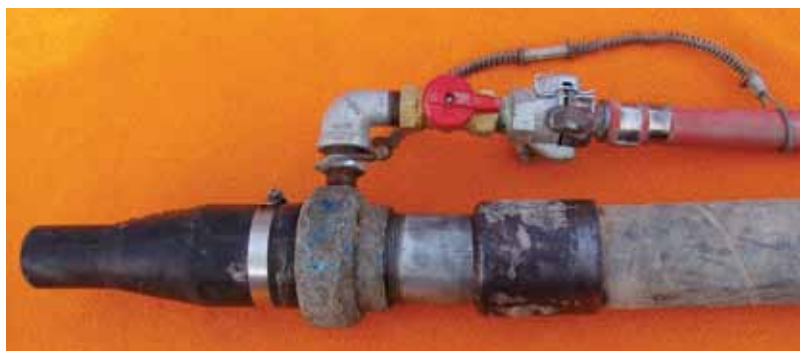
Fig 3: Two inch (50 mm) pipe thread acts as nozzle coupler
