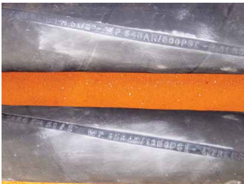
Fig 1: Top hose has a working pressure of 800 psi (5.5 MPa), which is underrated for shotcrete placement. The 1250 psi (8.6 MPa) pressure of the lower hose may be acceptable
