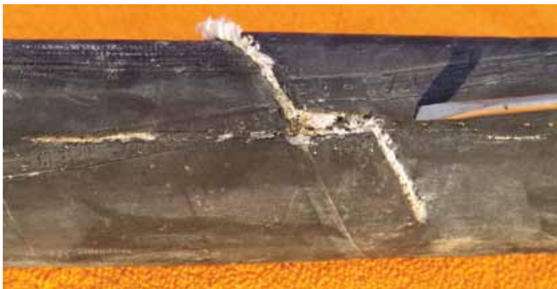
Fig 6: Interference with a foreign object caused this preventable failure
