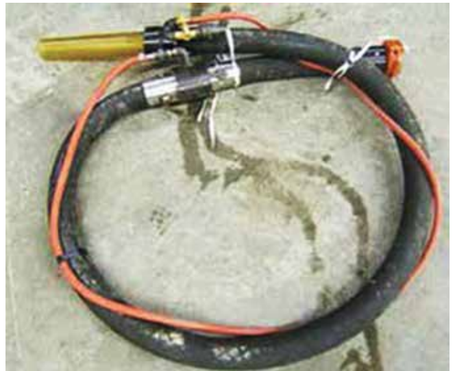
Fig. 10: Hydro-mix nozzle for dry-mix shotcrete (from Hutter, 2014)
