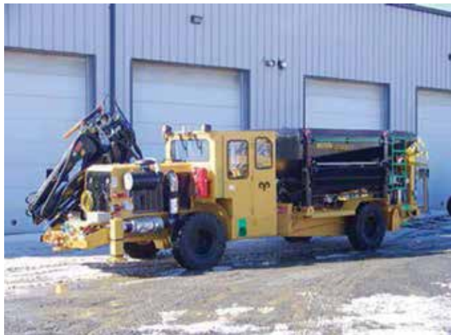
Fig. 6: Bulk dry shotcrete hauler/sprayer
