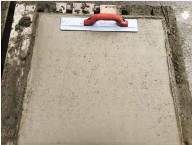
Fig. 10: Synthetic fiber mixture WSF finished with a magnesium trowel
