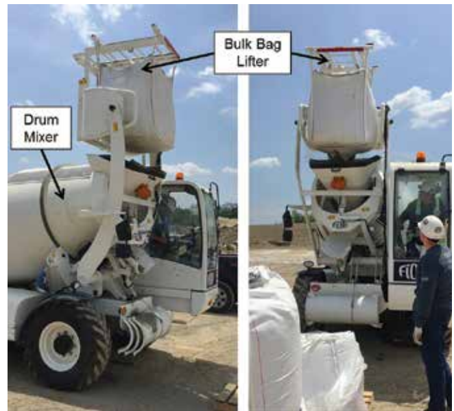
Fig. 5: Mobile self-loading mixer with bulk bag lifter
