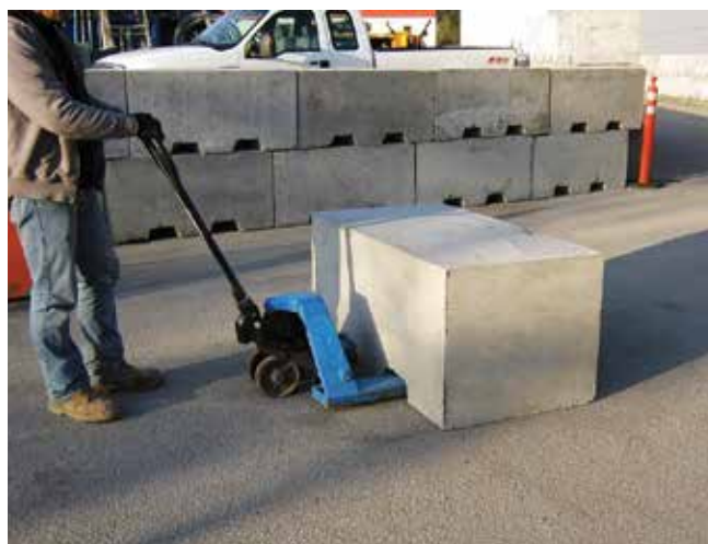
Fig. 10: Rebound and waste shotcrete cast onsite into useable retaining wall and barrier blocks, further contributing to the sustainability of shotcrete
