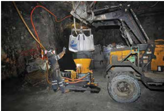
Fig. 8: Bulk pre-packaged tote bag with hopper hood
