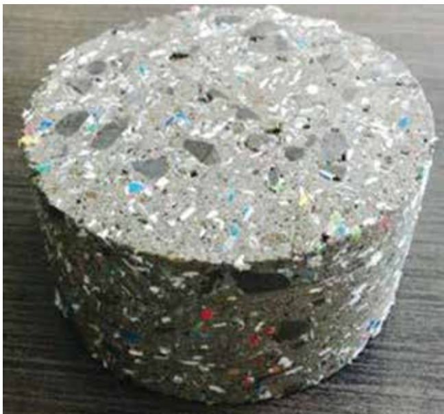
Fig. 7: Shotcrete core containing shredded recycled plastic 14
