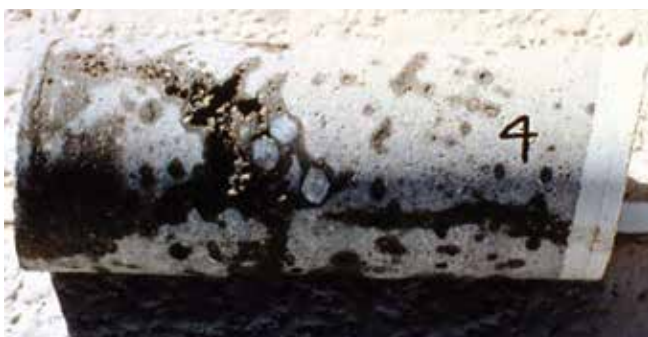
Fig. 3: Visual inspection of cores extracted from structures with unusual cracking or leaking can help to reveal improper shooting techniques or poor materials. All concrete has some degree of void or less than perfectly consolidated materials. Using an ACI Certified Nozzleman and crew that works well together to avoid inclusion of rebound is critical
