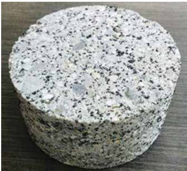
Fig. 8: Shotcrete core containing recycled rubber beads 14
