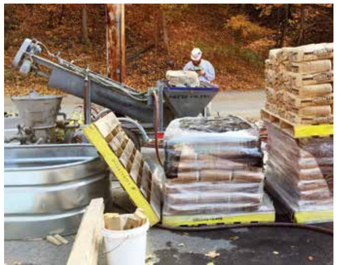
A typical setup used in dry-mix process refractory installations with a rotary gun and an auger-type pre-dampener for gunning dry prepackaged refractory material
