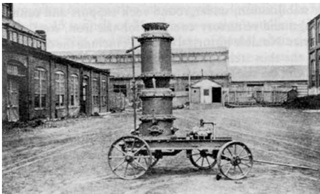
Fig. 1: Original double-chamber gun developed by Carl Akeley in 1907
