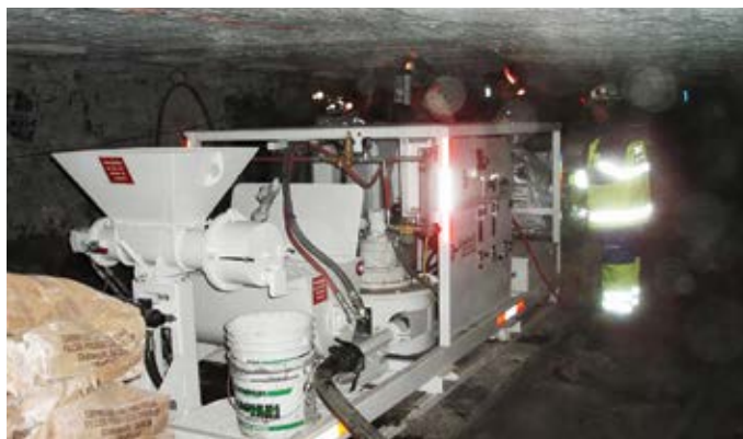
Fig. 3: Squeeze pump underground
