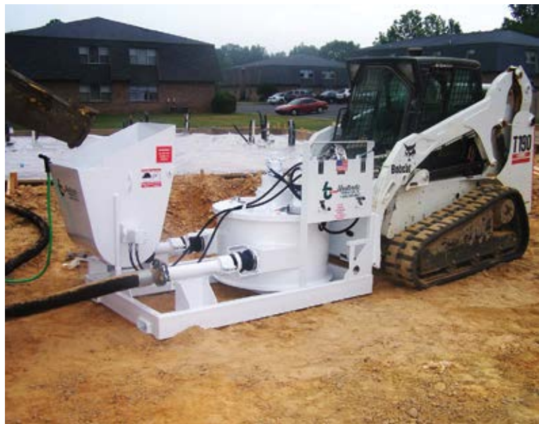
Fig. 2: Squeeze pump foundation pouring
