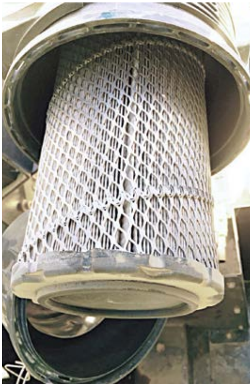
Fig. 3: A visual inspection can easily identify dirty air filters
