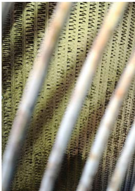
Fig. 6: Cooling fins clogged with dirt and oil area common cause of overheating
