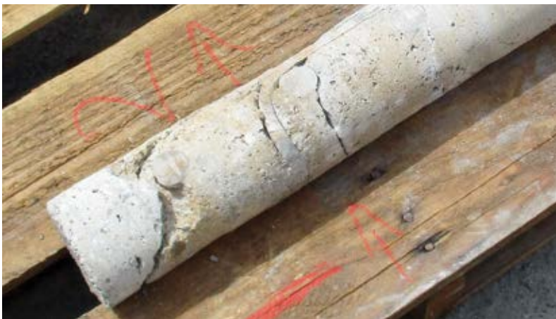
Fig. 7: Irregularities in one of the cores
