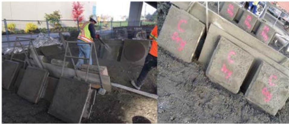
Fig. 3—Shotcrete test panels were shot by an ACI Certified Nozzlemaster for both wet-mix shotcrete (left) and dry-mix shotcrete (right).
