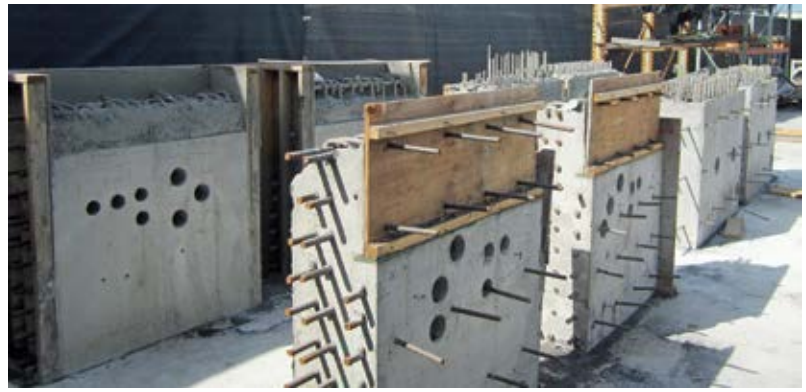
Fig. 3: Preconstruction test panels have been stripped, cored, and inspected
