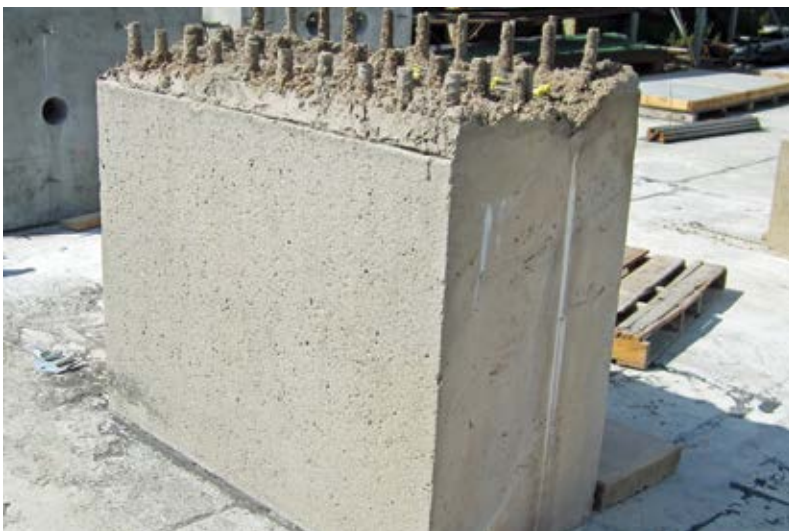
Fig. 8: Lightweight shotcrete mockup panel
