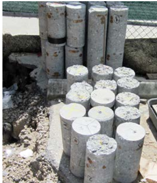
Fig. 4: Cores taken from thick wall preconstruction panels
