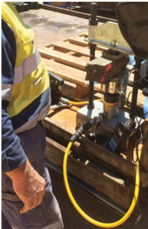
Fig. 1: Setup for beam end test
