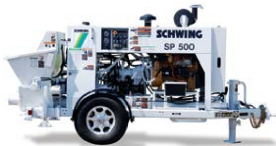
Fig. 5: The SP 500 is available with a Tier IV CAT diesel for low emissions operation in California
