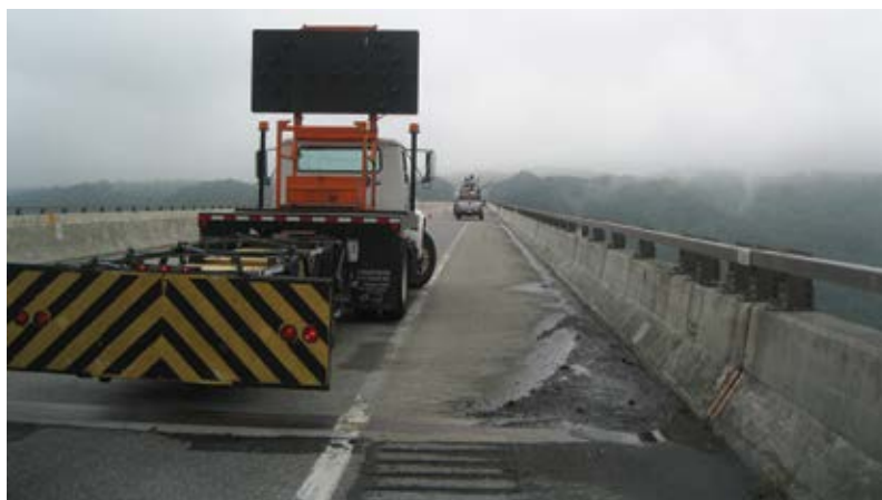
Fig. 3: Crash truck with impact attenuator and mounted arrow board, for a lane closure on a four-lane highway bridge in West Virginia
