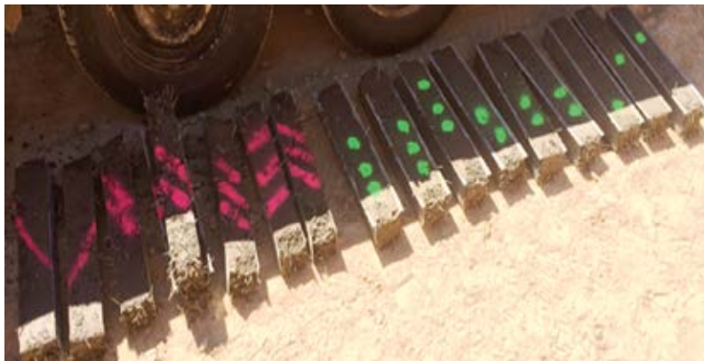
Fig. 2: Beams prepared to test early-age strength development
