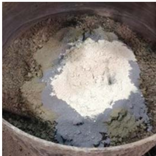
Fig. 1: Glass powder from crushed bottles (white), silica fume (gray), and cement
