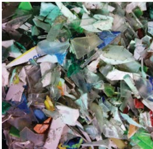
Fig. 3: Plastic aggregates (0.04 to 0.2 in. [1 to 5 mm]) from crushed plastic containers
