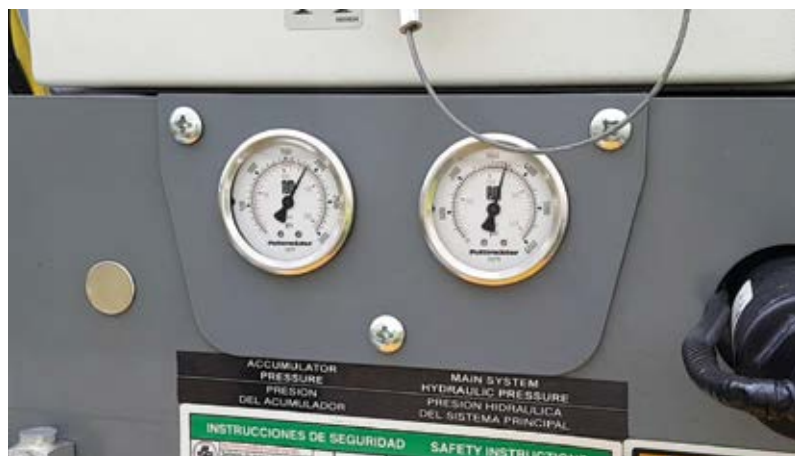
Fig. 5: Using hose only, this pump was pressuring out at 4600 psi (32 MPa) in the hydraulic system, or 1130 psi (7.8 MPa) on the concrete. Replacing 50 ft (15 m) of hose with pipeline lowered pressure to 3400 psi (23 MPa) in the hydraulics, or 835 psi (5.8 MPa) on the concrete
