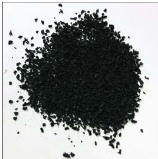
Fig. 4: Rubber aggregates (0.04 to 0.12 in. [1 to 3 mm]) from shredded tires
