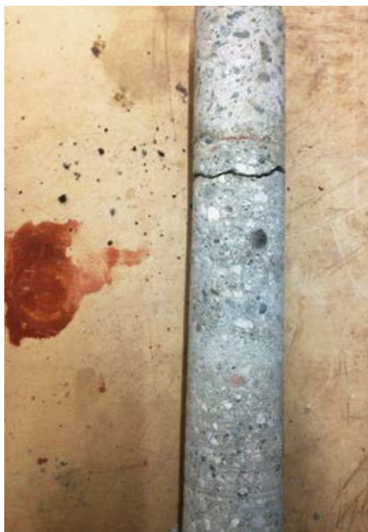
Fig. 4: A core taken from an in-place test panel. Note near the top is a faint red line—this is the tile layer seen in previous photos. In the 13 in. (330 mm) thick overhead section, ACI Certified Nozzlemen were able to achieve a solid bond without any separation between the new shotcrete and existing material. Due to the length of the core, it was not possible to drill through the length without breaking during the extraction
