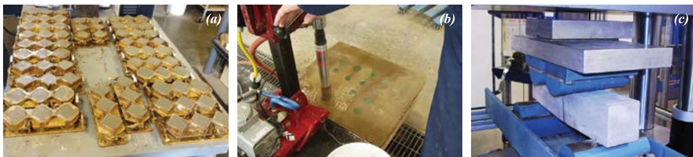
Fig. 1: (a) Compressive strength of mortar cubes; (b) cylinder coring; and (c) flexural strength testing of shotcrete beam with fibers
