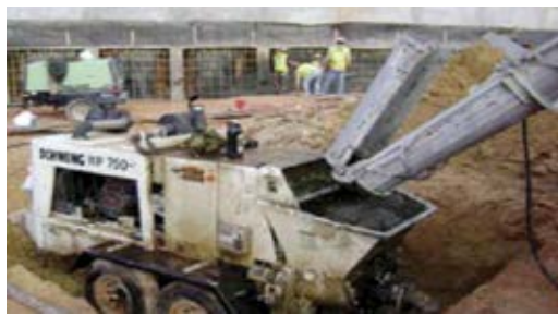
Fig. 14: Schwing 750 trailer pump setup for easy maneuvering in and around the jobsite can be reduced down to a 2 in. (50 mm) hose for shotcrete work or up to 5 in. (125 mm) for concrete pumping
