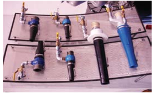
Fig. 11: Wet-mix shotcrete nozzle setups have a minimum of 3/4 in. (20 mm) air line running into them with 8 to 16 small 1/4 in. (6 mm) air holes in the air ring for maximum material velocity. Accelerator is introduced into the air stream at the nozzle and is driven into the material by the air flow (much like the dry-process water ring). The nozzle setup at the far right has an inner material ring and outer air ring. This nozzle needs the air volume to swirl the material coming out of the nozzle tip. With the separate accelerator port, the air volume is crucial to mix it into the material as it swirls out the tip. If the air flow is low, only the outside of the swirled material will have the accelerator in it (this nozzle is a newer version of the early technology)
