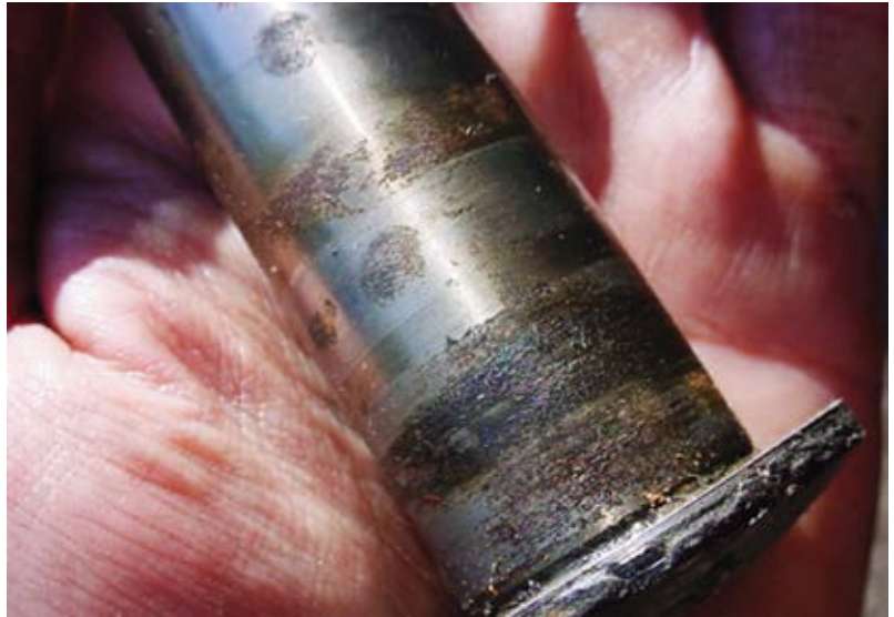
Fig. 1: Unnecessary corrosion and wear on critical bearing surface is likely caused by improper grease application
