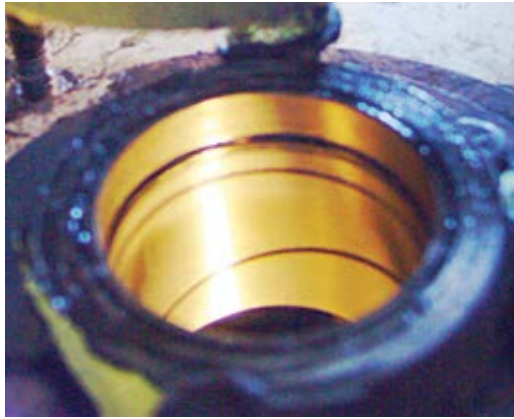
Fig. 3: Properly lubricated shaft bearing at 3000 hours
