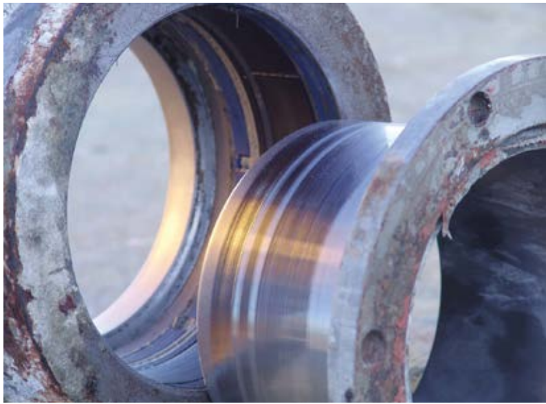
Fig. 5: Properly lubricated outlet bearing assembly at 3000 hours displays no visible wear
