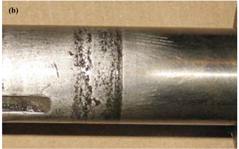
Fig. 4: (a) Note tight conditions within sealed bearing assembly; (b) bearing shaft showing significant corrosion and wear
