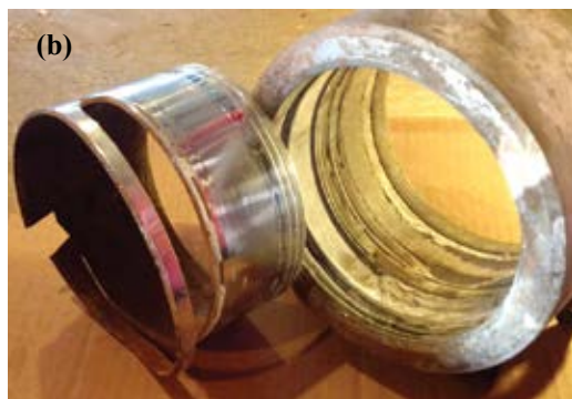
Fig. 6(a) and (b): Swing-tube shaft and outlet bearing assembly is totally destroyed at 1600 hours due to poor on-the-job lubrication practices. Note hardened concrete residue has clogged grease grooves of outlet housing on right
