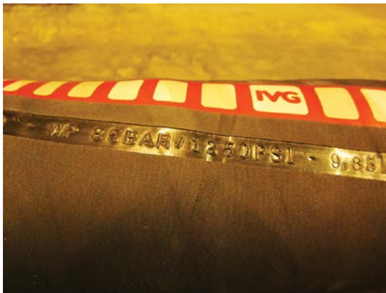
Fig. 1: All hoses should be labeled with maximum working pressure. This hose is labeled for a working pressure of 1250 psi (8.6 MPa)
