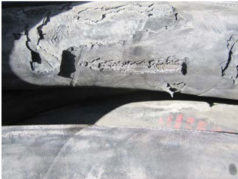
Fig. 2: The jacket on this hose has been damaged enough to expose the reinforcing cables, compromising the pressure capability of the hose. This hose needs to be replaced immediately
