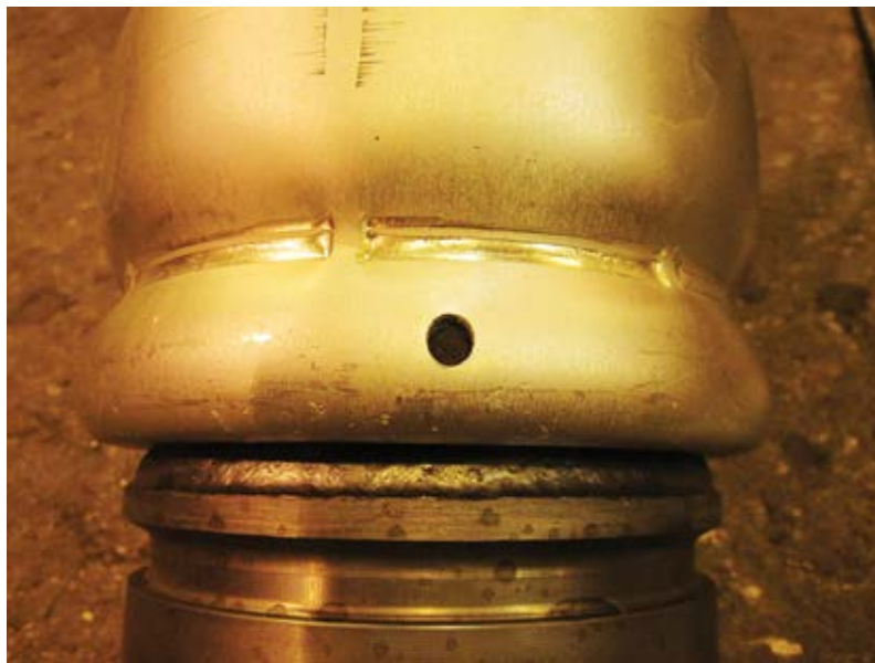
Fig. 3: Many hoses have a sight hole so you can check if the hose is seated all the way to the end of the ferrule and is not pulling out
