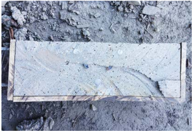
Sawed side of shotcrete test panel shot with multiple layers
