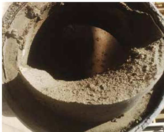
Fig. 3(c): Hardened buildup restriction inside the S tube is caused by worn wear components
