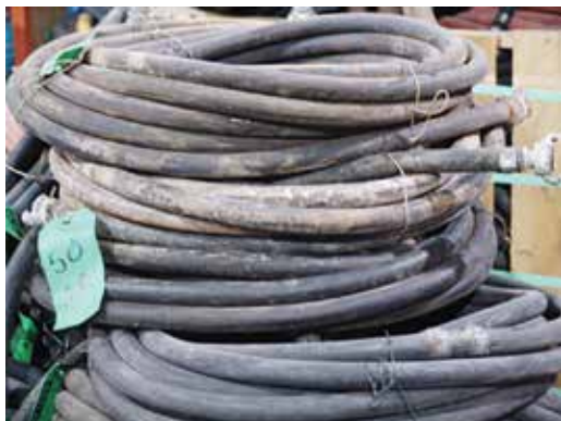
Fig. 7: Air supply line diameter is critical to maintaining adequate nozzle velocity
