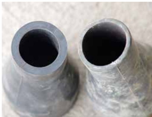
Fig. 6: Worn tip (right)
