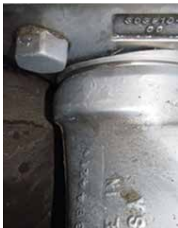
Fig. 3(a): Worn wear components will allow moisture to be squeezed from the mixture during pumping
