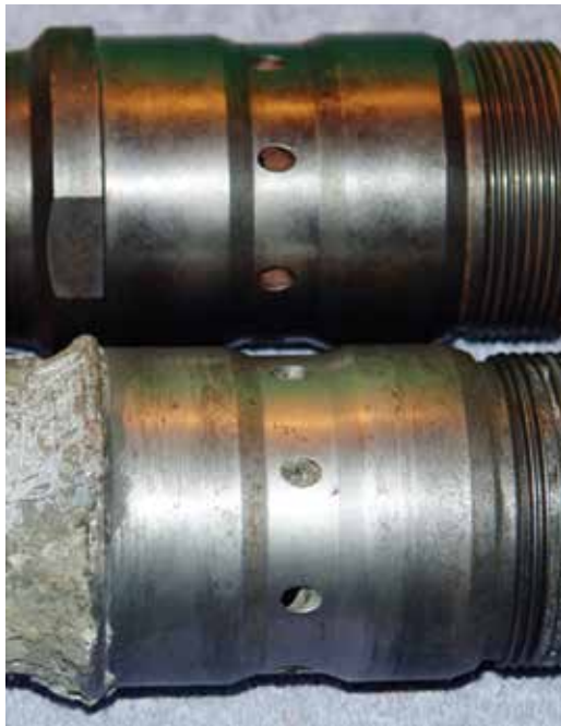
Fig. 4: Note plugged air ring port on lower nozzle. A single plugged port will dramatically reduce in-place compaction/consolidation quality
