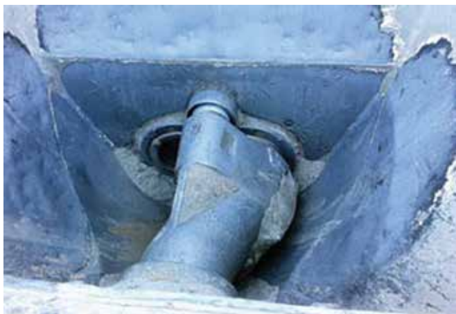
Fig. 1: Missing auger cannot provide adequate cylinder filling. Uneven nozzle flow will affect nozzle placement quality
