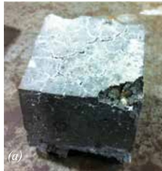
Fig. 7: (a) Expansion of a mixture close to the expansion line; and (b) expansive mixture compare to a stable mixture
