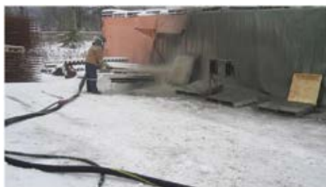
Fig. 1: Shooting test panels above ground in winter conditions
