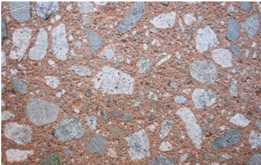
Fig. 5: Rapid-strength-gain dry-mix shotcrete modified with red pigment
