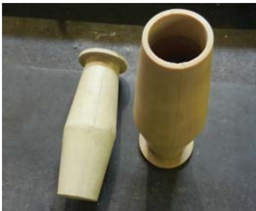
Fig. 8: Dry-mix nozzle liner with interior steps/ridges
