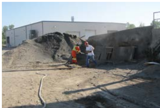
Fig. 2: Shooting test panels and end beams on surface in summer conditions
