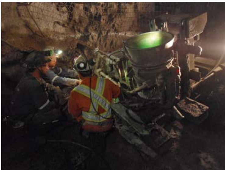
Fig. 4: King representative working with mining personnel to perform maintenance on a dry-mix shotcrete machine
