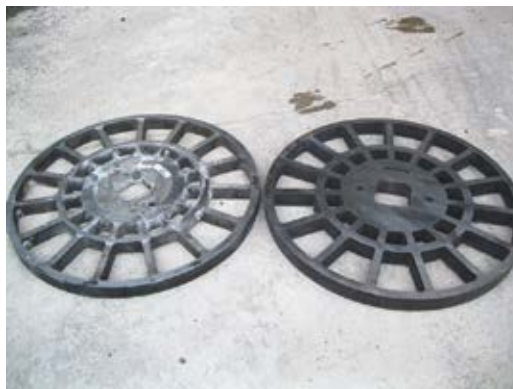
Fig. 2: Worn plate (left), new plate (right)
