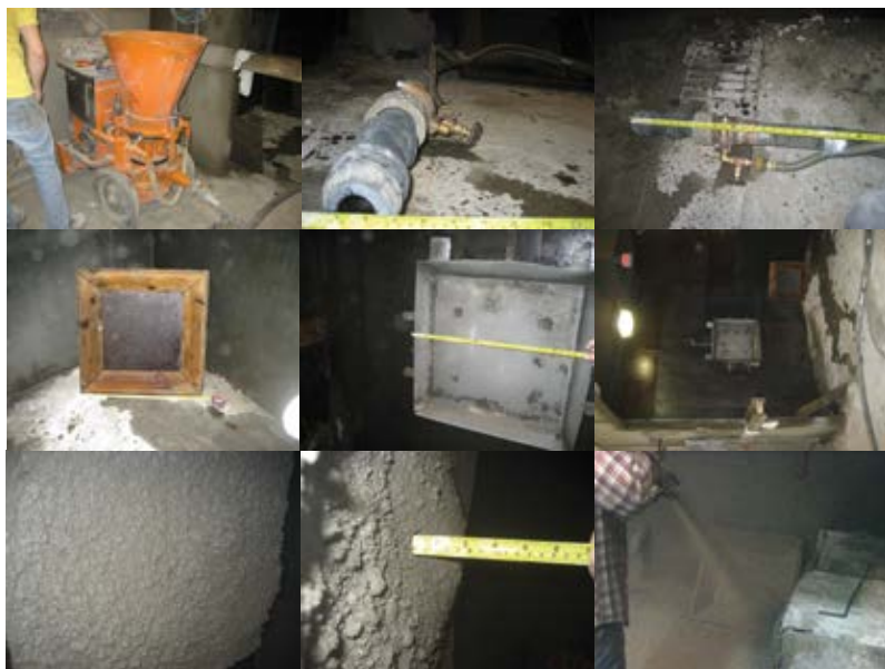
Fig. 2: Aliva 246, material and operator on scale (top left), double bubble nozzle (top middle), short hydromix nozzle assembly (top right), shotcrete panels (middle left), rebound panel (middle middle) and shooting area overview (middle right), fresh control mixture on rebound panel (bottom left), measuring buildup (bottom middle), shooting control mixture panel (bottom right)
