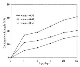
Fig. 4: Development of compressive strength of concrete with different w/cm (RHA content = 10%) (Originally from Fig. 2-4 of ACI 232.1R-00 [Zhang and Malhotra]) (Note: 1 MPa = 145 psi)
