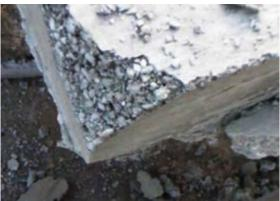
Fig. 1: Poor placement techniques have produced sand lens or encased rebound trapped within test specimen
