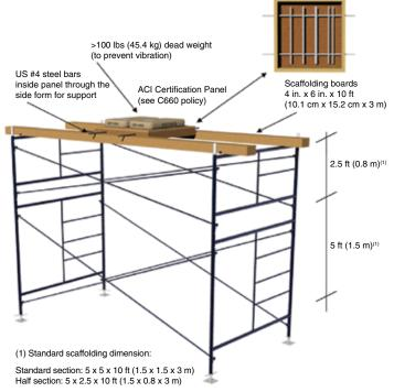
Typical ACI overhead Test Panel setup
