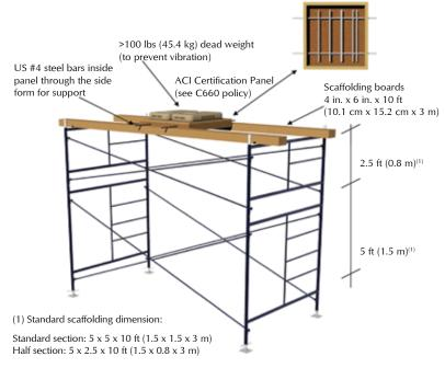
Fig. 1: Overhead standard set-up—ACI Shotcrete Nozzleman Certification
