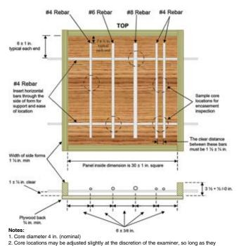
remain along the axis of the reinforcing bars, and at least three bar intersections are covered
