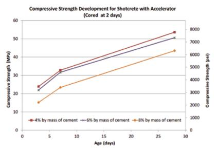
*Fig. 2: Compressive strength development for shotcrete; cores taken at 2 days of age*
