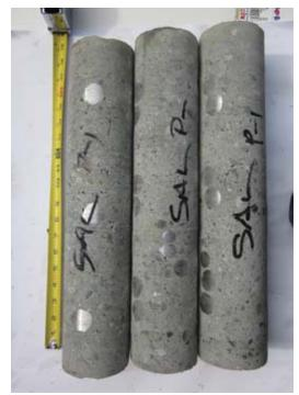
*Fig. 3: Cores retrieved from Type 1 preconstruction test panel*
