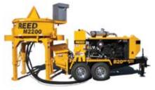
REED's newest MixerPump Combo was designed specifically for shotcreters who need both a powerful, high-pressure shotcrete pump and a fast, robust mixer. A 160 hp (119 kW) Cummins diesel motor and twin variable-displacement hydraulic pumps on the B20HP-PP "Power Pack" provide enough power to drive both the 20 yd<sup>3</sup>/h (15 m<sup>3</sup>/h) 2113 psi (14.6 MPa) B20HP Pump and direct hydraulic drive 1-Ton M2200 model Mixer.
