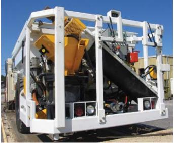
*Hybrid-Wet*<sup>®</sup> *Shotcrete Carrier with Aliva 257 and mixing chamber*
