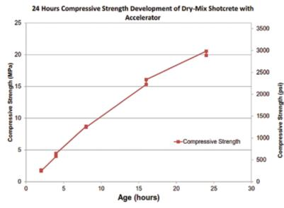
Fig. 4: Early-age compressive strength when tested with end beam tester
