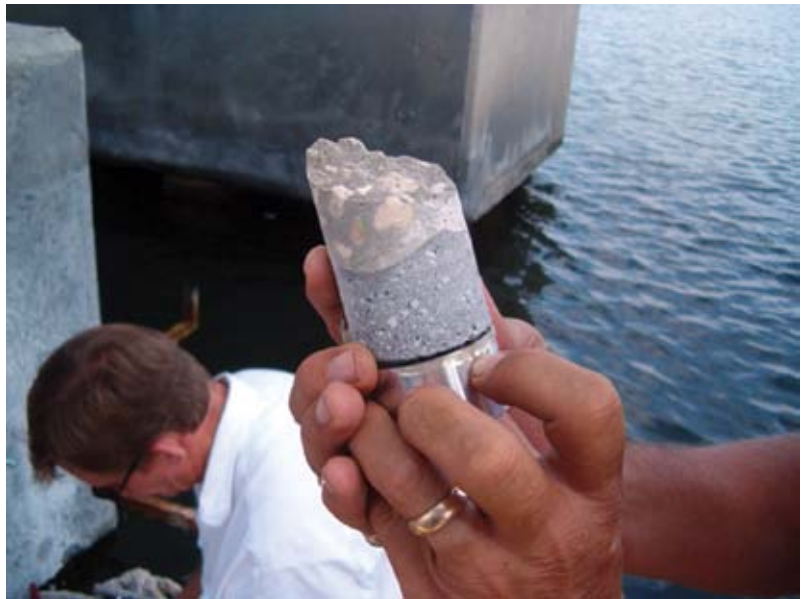
Pullout test showing core failure in substrate
