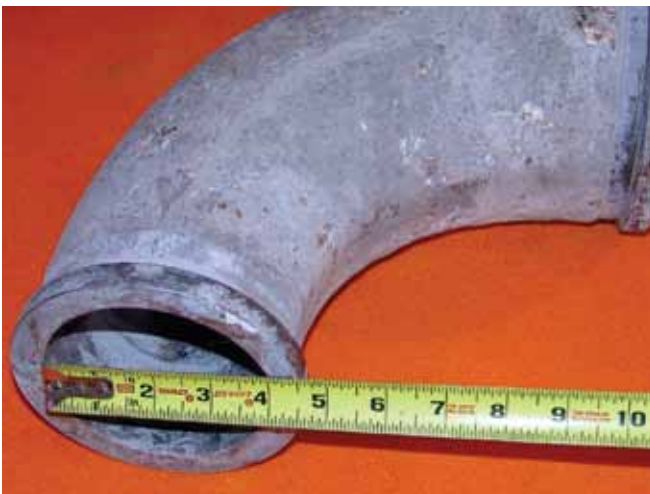
Fig. 3: Elbow A (left) displays a 4 in. (101 mm) interior diameter. Elbow B (right) measures 4-5/16 in. (109 mm)
