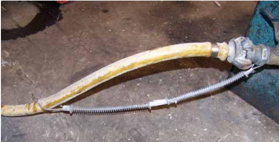
Use of whip checks with pneumatic tools at each connection point
