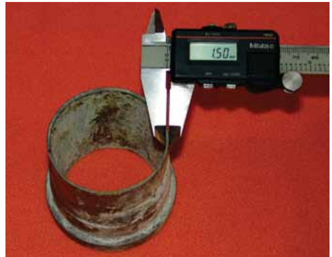
Fig. 2: Reducer A (left) displays acceptable wall diameter. Reducer B (right), with a wall thickness of 0.06 in. (1.5 mm), illustrates a burst hazard
