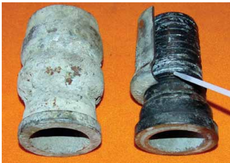
Fig. 6: 2 in. (50 mm) hose couplers create a unique safety risk. Thinnest area of coupler is hidden within collar (pointer), making external wall thickness validation impossible. Saw cutting revealed insufficient wall thickness for any 2 in. (50 mm) coupler, which measured 1/8 to 5/32 in. (3 to 4 mm) oversized ID. Note: Raised-end component shapes created challenges using conventional machinist calipers to determine wall thickness
