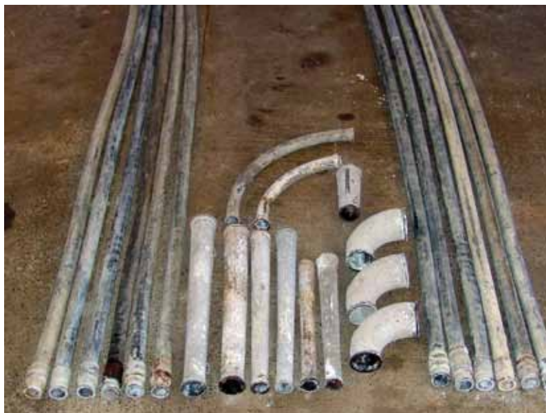
Fig. 5: Placement system components prior to saw cutting
