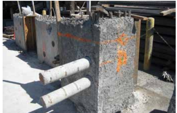
Fig. 5: Example of a completed job-specific test panel. Drilled cores have been removed to evaluate encapsulation of reinforcing bar
