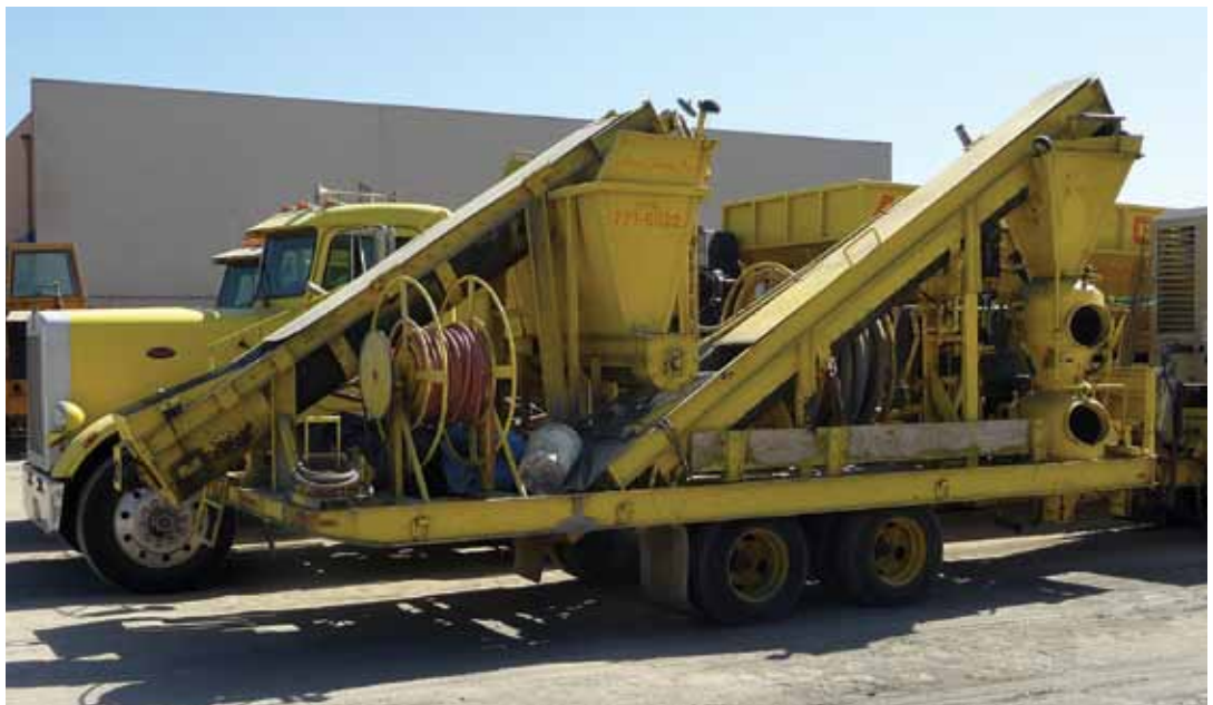
Fig. 8: Rig with mobile mixer has over 40 ft (12.2 m) of auger mixing
