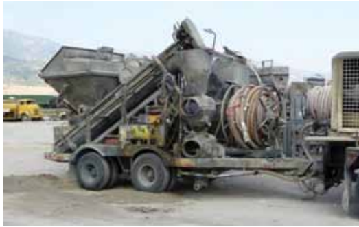
Fig. 5: Contractor-built gunite rig using auger mixing
