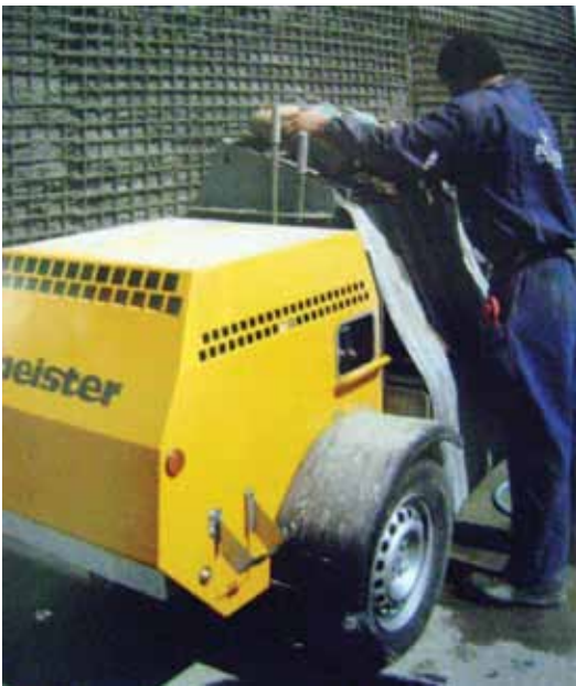
Fig. 2: The SP 13 high-pressure piston pump. The low profile gives the operator an unobstructed view of the work area and shooting area while making a batch of wet-mix concrete
