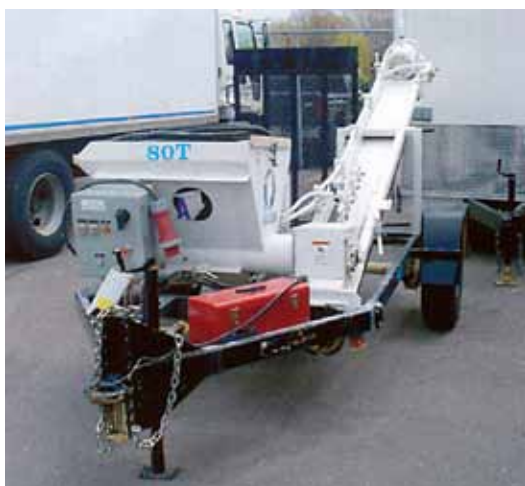
Predampener used in dry-mix shotcrete application
