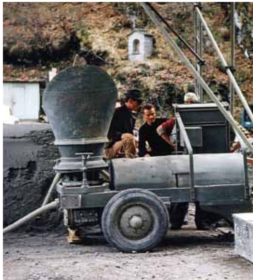
Fig. 4: American rotating-barrel gun (Jetcreter)
