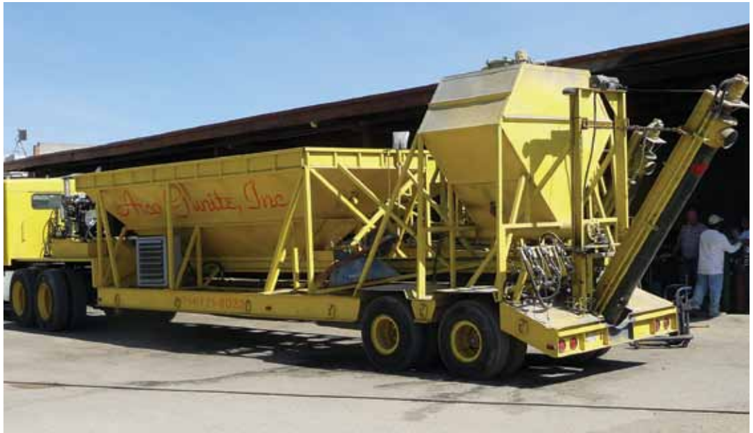
Fig. 7: Custom-built mobile mixer can deliver 17 tons (15.4 metric tons) of dry-mix material
