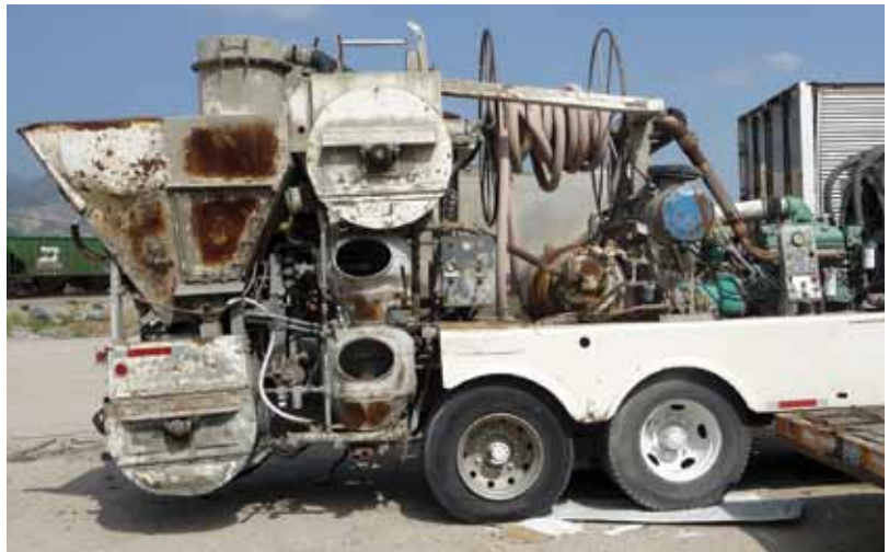
Fig. 2: View of the paddle mixer showing the double chamber gun
