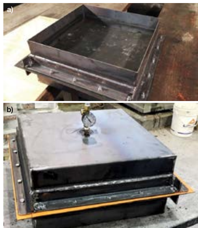
Fig. 5: (a) Testing frame from membrane side; and (b) from air input side
