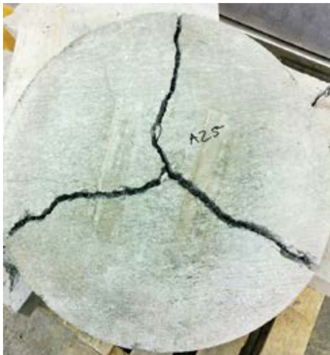
Fig. 2: Typical ASTM C1550 specimen (RDP) after testing
