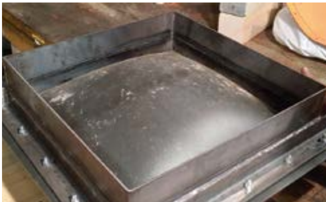
Fig. 9: Inflated membrane at 50 psi of air pressure
