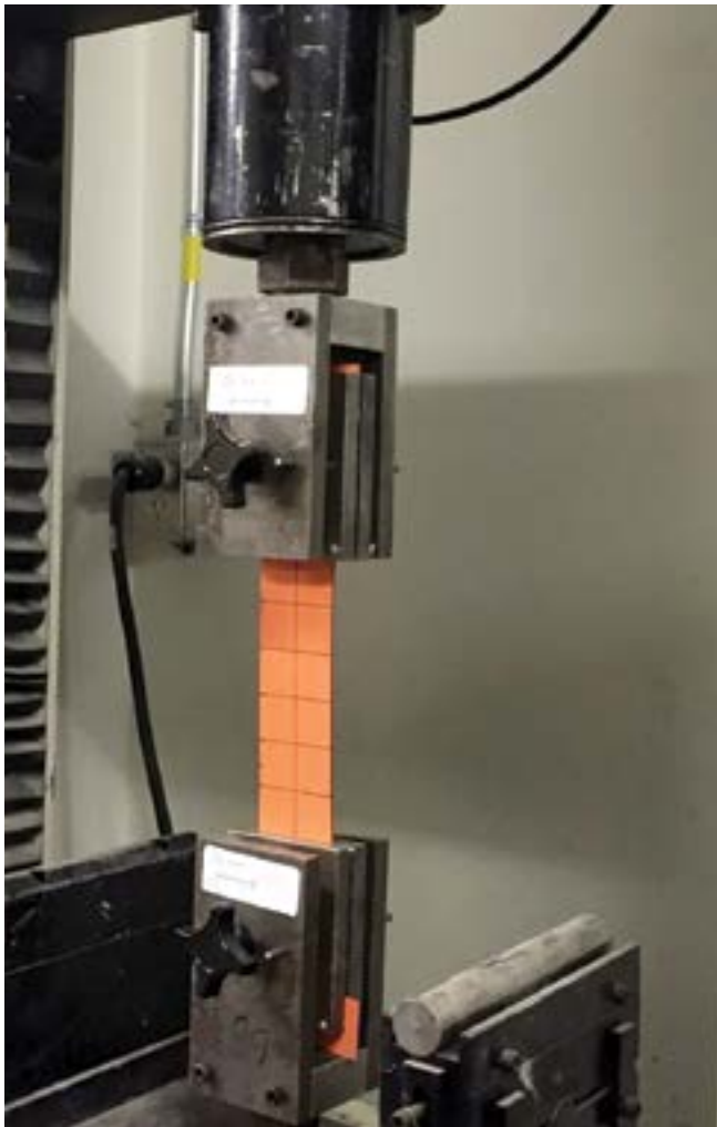
Fig. 6: Overall view of a membrane at the beginning of the test
