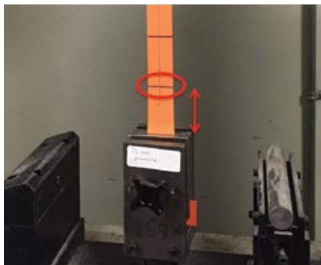
Fig. 10: Membrane slipping outside the clamping jaw for crosshead displacement of 14 in. (350 mm)
