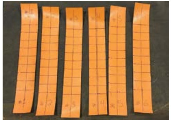
Fig. 7: Waterproofing membrane in strips before testing
