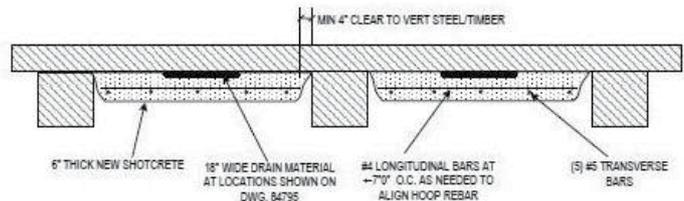
Note: 1. For Mat #1, center (3) #5 polyester resin bonded dowels to be embedded into the concrete curb between each set of timbers. [Depth of Embedment = 6" Length of Bar = 36" total]
