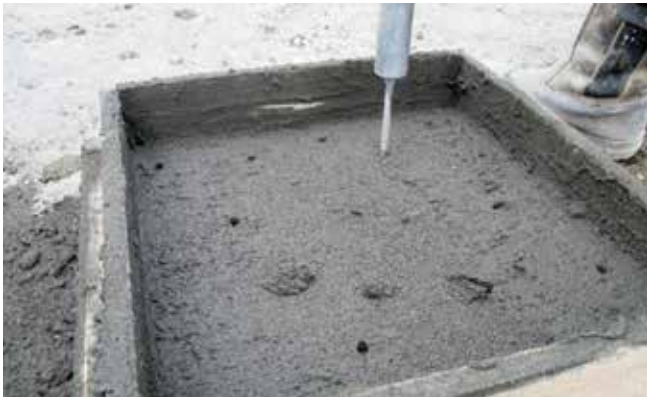
Fig. 12: Determination of initial and final set based on testing in accordance with ASTM C403/C403M
