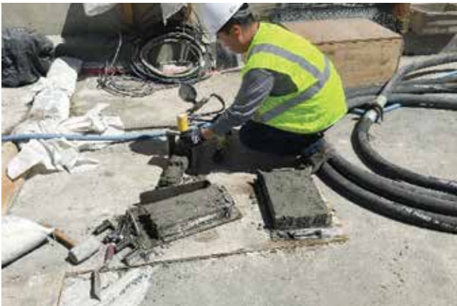
Fig. 13: Determination of early-age compressive strength based on testing in accordance with ASTM C116
