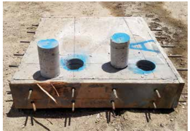
Fig. 2: Preconstruction test panel for cores approving nozzle men for project
