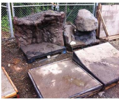
Fig. 3: Three-dimensional samples displaying the different textures were prepared for approval prior to production
